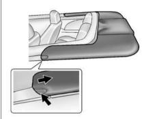
Grip the tonneau cover at the notch and pull back to release the tab on both sides.
