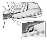
4. Insert the tab (1) under the trim (2) on both sides.
