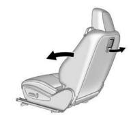
To access the rear seats, pull up on the latch on the rear of the driver or front passenger seatback. Fold the seatback forward.
