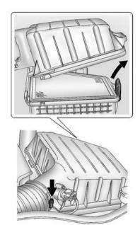
3.6L V6 Engine Air Cleaner/Filter Housing Shown (6.2L V8 Engines Similar)
