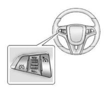
(On/Off): Press to turn the system on and off. A white indicator appears in the instrument cluster when cruise is turned on.
