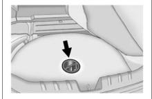
Turn the center retainer counterclockwise to remove the cover.
