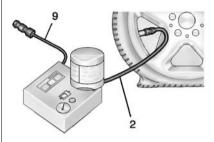
Attach the sealant/air hose (2) to the tire valve stem by turning it clockwise until tight.
