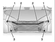
The upper (1) and lower (3) hooks on each side of the trunk opening are provided to attach the net.
