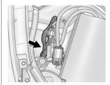
The electrical cord is on the passenger side of the engine compartment, next to the engine compartment fuse block for V6 models.
