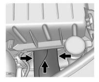
Press in on the tabs on the sides of the duct, and then push the duct rearward into the air cleaner/filter housing.
