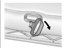
After the convertible top is completely raised, release the convertible top front latch from the lock position by pulling down and turning it clockwise.  Lock the convertible top front latch by pulling down and turning it counterclockwise, then push it up.
