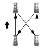
Use this rotation pattern when rotating tires of the same size installed on all four wheel positions.
