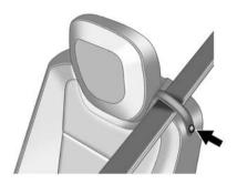
If the seat has a safety belt guide, and the safety belt is not routed through the guide, snap the guide around the belt webbing. Be sure the belt is not twisted. Adjust the seat, if the seat is adjustable, so you can sit up straight. To see how, see "Seats" in the Index.
