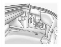
The rear compartment fuse block is on the right side of the trunk behind a cover. Remove the convenience net retainers, the rear sill plate, and the passenger side trim retainers, then swing the trim out of the way.
