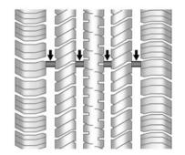
Treadwear indicators are one way to tell when it is time for new tires. Treadwear indicators appear when the tires have only 1.6 mm (1/16 in) or less of tread remaining. See *Tire Inspection on page 10-70* and *Tire Rotation on page 10-70*.
