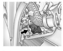
The instrument panel fuse block is on the end of the instrument panel, on the driver side of the vehicle. To access the fuses, open the fuse panel door by pulling out.
