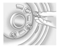
Remove all of the wheel nuts and place them in a dry, clean place to avoid getting dirt in the threads.
