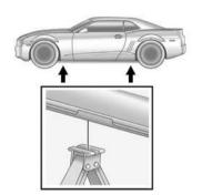
4. Position the jack lift head at the jack location nearest the flat tire. The location is indicated by a mark on the bottom edge of the vehicle. The jack must not be used in any other position.
