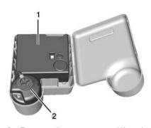
6. Remove the compressor (1) and the sealant canister (2).
