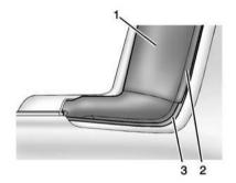
6. Push the edge (2) of the center of the tonneau cover (1) under the vehicle trim (3).
