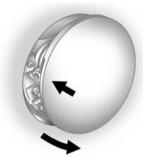
The fuel cap is behind a hinged fuel door on the passenger side of the vehicle. To open the fuel door, push and release the rearward center edge of the door. To unlock the fuel cap on vehicles equipped with a locking fuel cap, use the key provided with the Remote Keyless Entry (RKE) transmitter.
