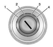
The ignition switch has four different positions.
