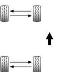
Use this rotation pattern if the vehicle has different size tires on the front and rear and they are non-directional.
