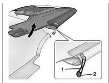
Fold the sides of the tonneau cover over. Attach the cord (1) at the front edge of the tonneau cover to the post (2) on the back seat rear panel on both sides.
