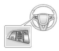
ৈ: Press to turn the system on and off. A white indicator appears in the instrument cluster when cruise is turned on.
