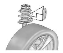
Due to low ramp angles on the ZL1 and Z/28, use care when loading the vehicle onto a flatbed carrier. Front spring spacers were provided for lifting the front suspension if more clearance is necessary when towing.
